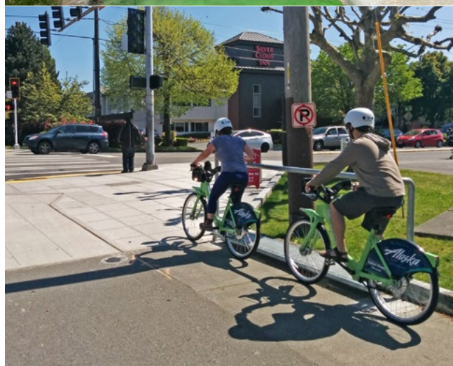
Bicycle lean rails installed within separated bike lanes in Charlotte, NC (top) and Seattle, WA (bottom)
