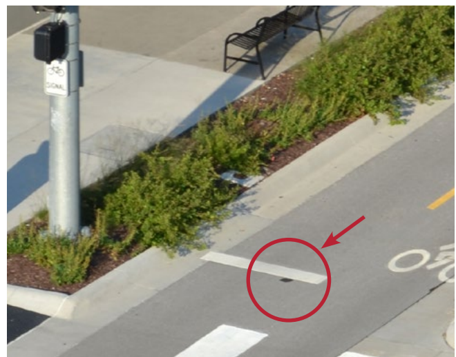
In-ground radar installation patch in Lincoln, NE. Ultimately, this system was deactivated and the signals reverted to fixed timing.
