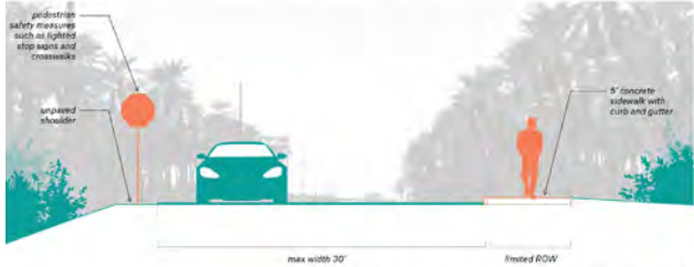
Typical Cross-Section: 5-foot Wide Concrete Sidewalk with Curb
