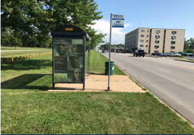
Figure 2: A bus stop island in a sea of grass. There is no meaningful access for a person with a disability.
