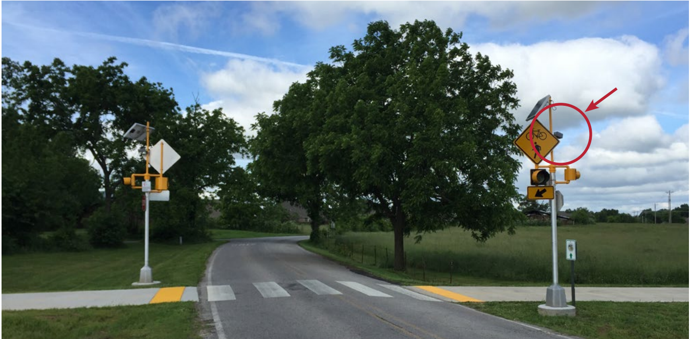
This microwave detector in along the Razorback Greenway in Northwest Arkansas activates a warning beacon when a trail user (pedestrian or bicyclist) is approaching the roadway crossing.
