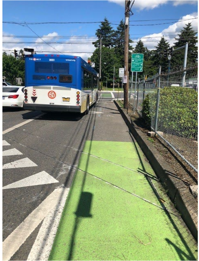
Parallelogram Loop Detector Configuration in Portland, Oregon detects bicyclists and vehicles entering this mixing zone. This location puts in a locking call and extended green for bicyclists. (Credit: Oliver Smith)
