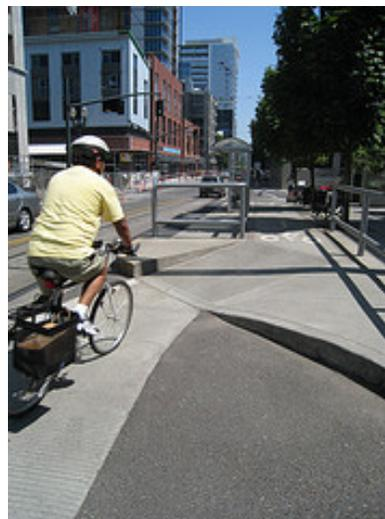
*At this sidewalk detour in Portland, pavement markings and railings differentiate between cyclist and pedestrian zones.*
