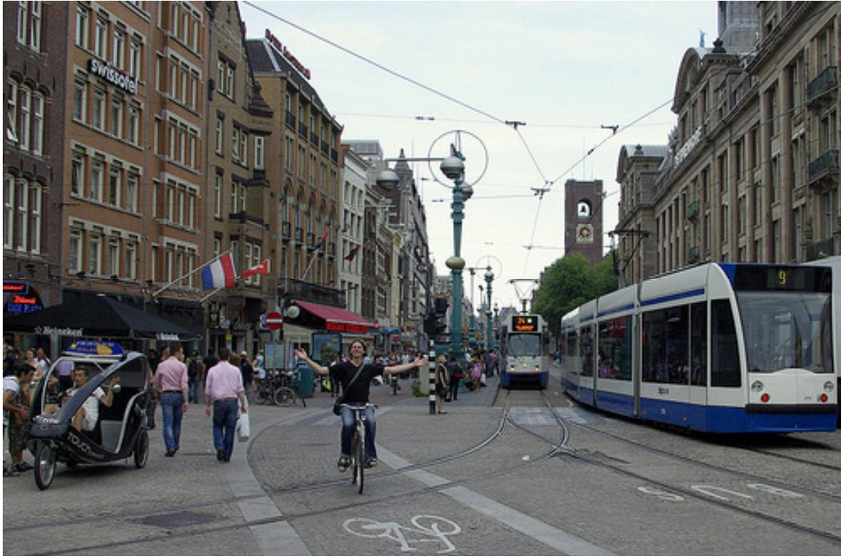
*This photo from Amsterdam illustrates many of the international best practices identified above: spatial separation of the cycle track from tram tracks, center-running tracks and platforms, separation of bicyclists and pedestrians, clear pavement markings directing cyclists, and near-perpendicular track crossing angles. Source: <http://www.flickr.com/photos/anw-fr/2744645044/> (used with permission)*
