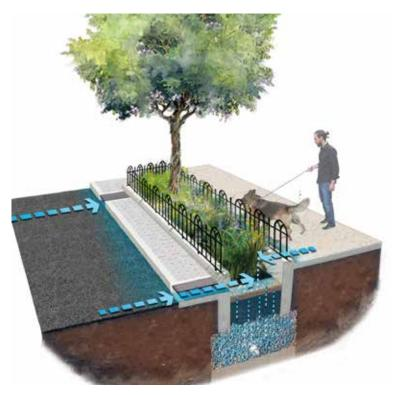
Figure 12. Stormwater Planter
