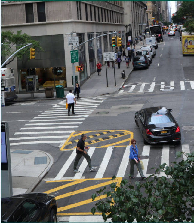
ABOVE LEFT: a passenger vehicle turns left at the intersection of two one-way streets, steering around a rounded corner apron with diagonal speed humps. Credit: NYC DOT. ABOVE RIGHT: an example of a square corner apron outlined with speed bumps. Credit: NYC DOT.
