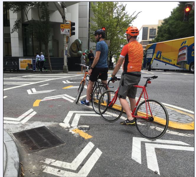
ABOVE LEFT: The corner design treatment applied at 10th NW and Brady. The apron is defined by a mountable curb with a significant vertical component. ABOVE RIGHT: The corner design at Peachtree Center and John Portman. BELOW: Two bicyclists queuing behind the mountable corner apron at Peachtree Center and John Portman.
