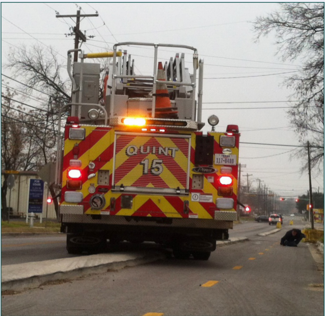
Austin Fire Department “Quint” testing a mountable curb profile. Photo: City of Austin.
