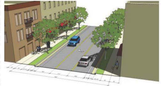
In the illustration above from the Connect Atlanta Plan , the number of travel lanes is reduced from four lanes to three lanes. With one fewer lane, the extra street space can be used for expansion of sidewalks, street trees, or bikeway facilities. The addition of the center turn lane helps preserve vehicular capacity for the outside travel lanes while also improving safety for vehicles making left turns, either midblock or at intersections. This type of street design strategy was used frequently with this study to create space for bikeway facilities.
