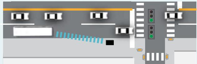
Signal controller detects bus; extends current green phase
