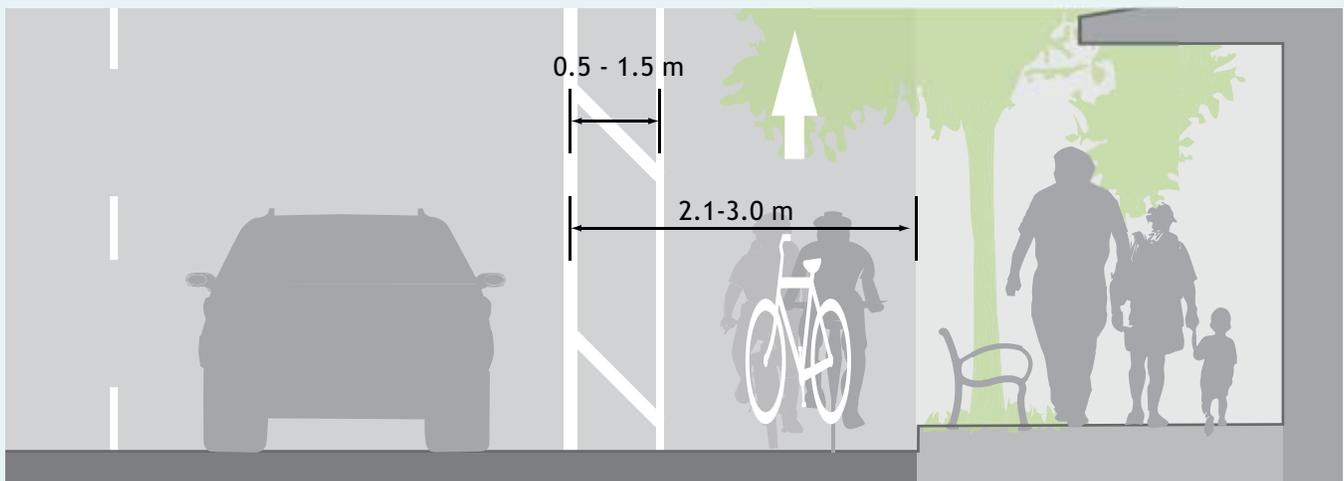
Standard width of a bike lane and associated buffers is 2.1 - 3.0 m.
