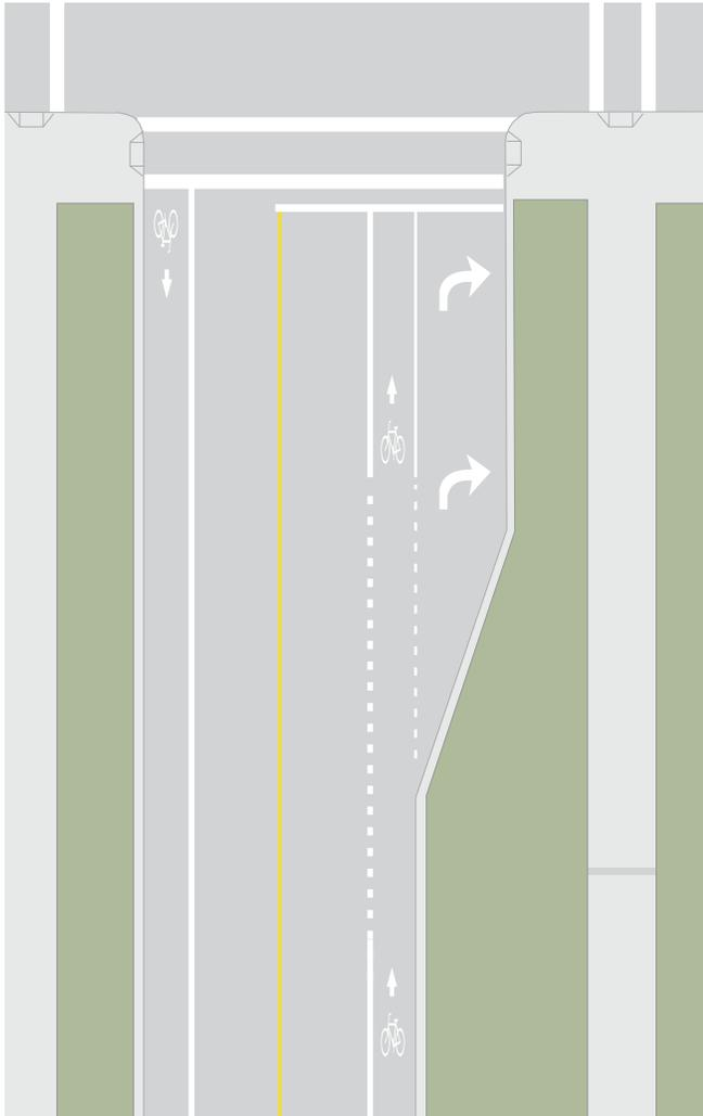
When a through lane transitions into a right turn lane, use dashed lines to offer bicyclists flexibility in negotiating the transition area.
