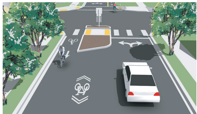
Figure C26. Traffic diverters allow through bicycle movements while restricting motor vehicle traffic.
