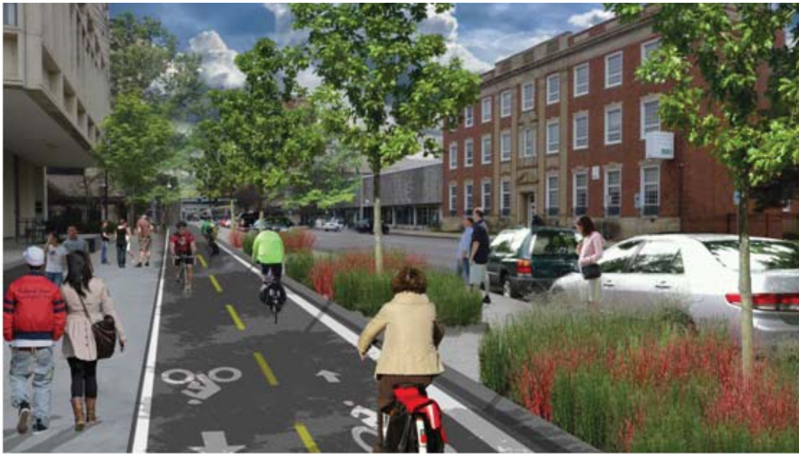
For a cycle track in Lincoln, NE, Alta identified an opportunity to capitalize on additional project funding from the City's Watershed division by designing stormwater infiltration planters in the buffer between the cycle track and parallel parking and in pedestrian refuge islands at each intersection. The project is currently being bid for construction.
