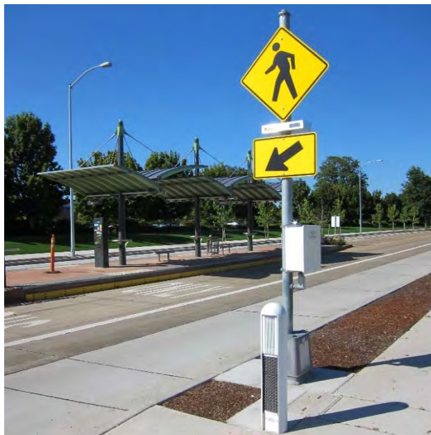
Figure 99: Rectangular rapid flashing beacons help to identify important pedestrian crossings.
