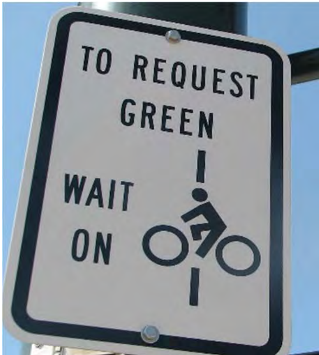
Figures 82 and 83: Signage and pavement markings direct bicyclists to use the pavement detection loop to activate a traffic signal.
