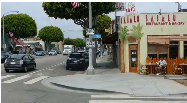
Figures 71 and 72: These curb extensions pictured above support pedestrian mobility in busy commercial districts. .
