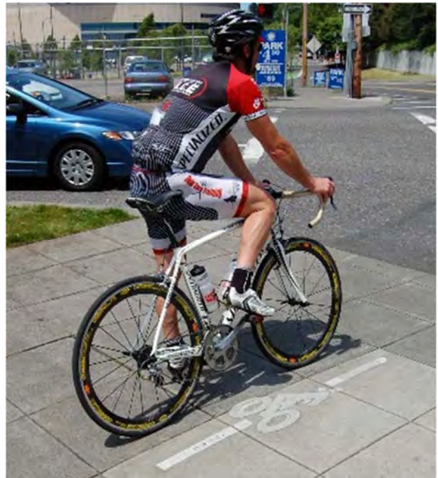
Figures 82 and 83: Signage and pavement markings direct bicyclists to use the pavement detection loop to activate a traffic signal.
