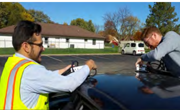
Figure D.7 A PEO/PA attaching LPR cameras to a car roof with magnets
