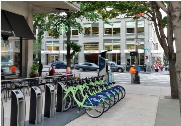
Dock-based station: uses steel plates and electromagnetic docking points (Seattle Pronto)
