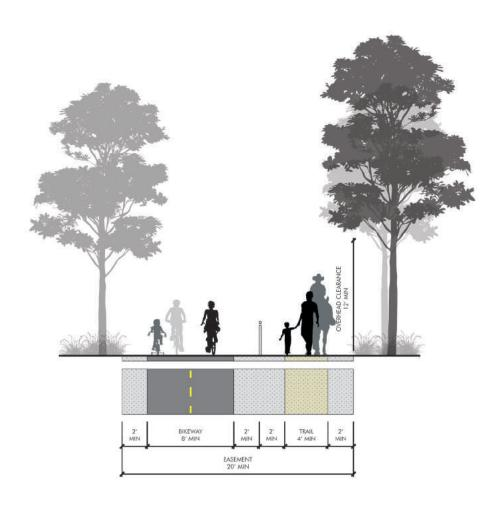
Typical Section: Class I Bikeway w/ Side Trail and Fence, Constrained
