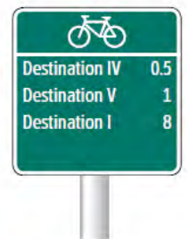
C Confirmation sign After decision points, confirmation signs reassure cyclists of their direction and confirm additional destinations reached along that route.
