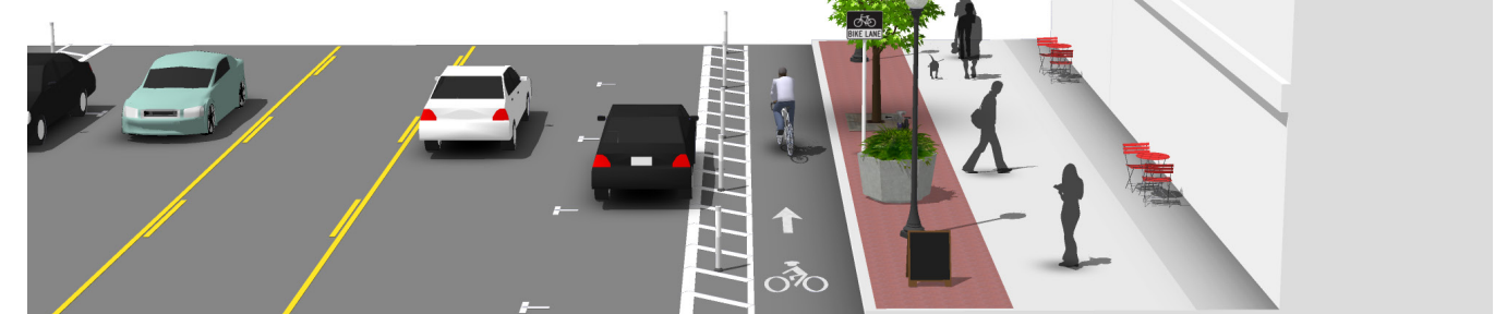
Paint and bollard street-level protected bike lane retrofit:
