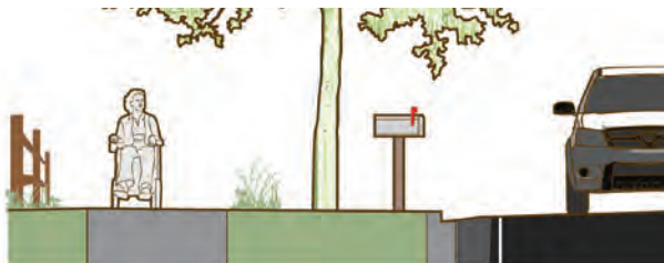
Figure 4-15. Sidewalks on roads with curbs may feature an unpaved or paved furnishing zone separation (left), or may be constructed with curb and gutter, immediately adjacent to the roadway (right). Offering separation from the roadway is preferred in most areas for user comfort and design flexibility at intersections.
