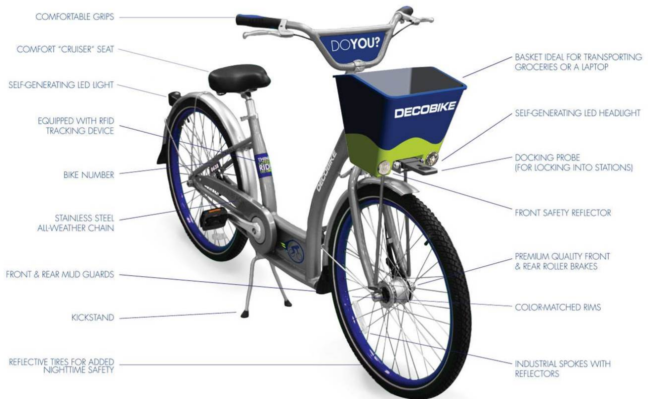
Figure 11: Safety Features of a Typical Bike Share Bicycle (DecoBike, Miami Beach)
