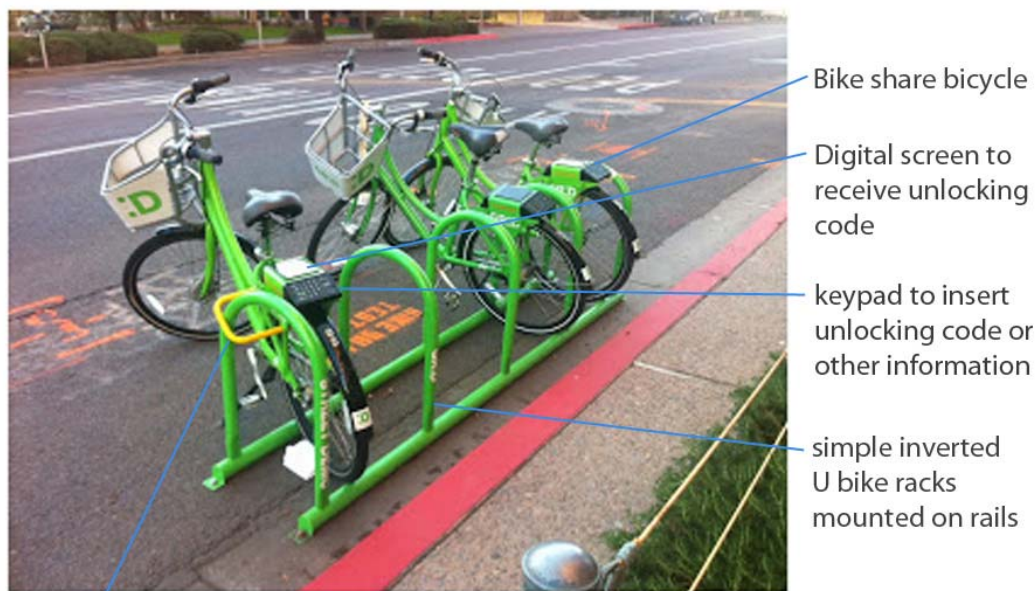
Figure 4: Elements of a 4 th Generation Stationless Bike Share System
