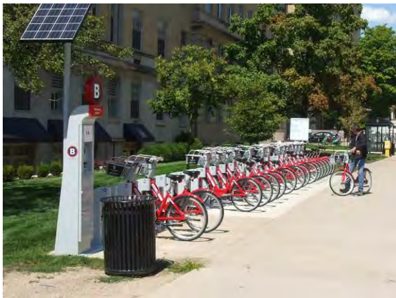
Dock-based station: utilizes steel plates and electromagnetic docking points (Madison B-Cycle)
