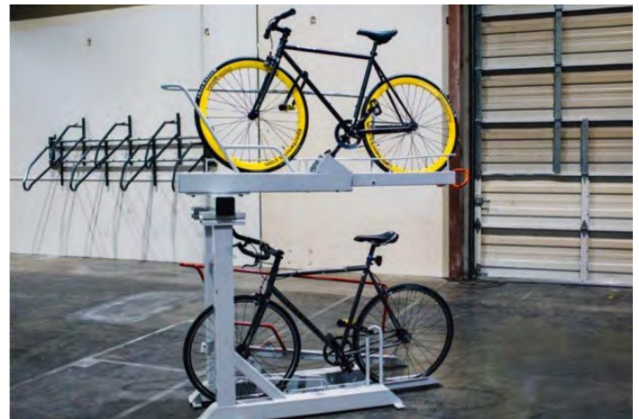
If multi-level racks are desired, the top level should provide a mechanical or hydraulic assist to help people lift their bike. Recognizing that most people prefer to use the bottom level, the bottom tier of the Josta Double Parker System has two spaces for ever one above.
