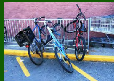
Wheel bender racks are poorly designed, allowing bicycles to easily tip over and appear disorganized.
