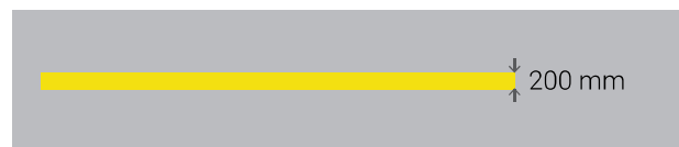
Figure 4.16 – Yellow Contraflow Lane Line
