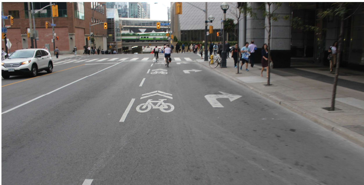
Figure 6.45 – Example of Mixing Zone, Toronto
