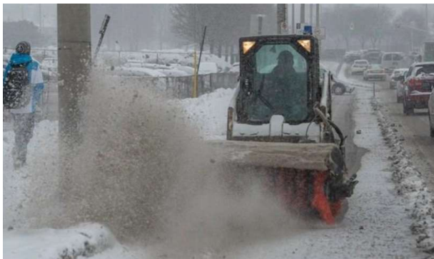
Figure 10.24 – Winter Maintenance Vehicle with Brush Attachment, Hamilton
