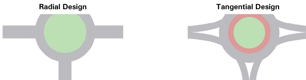
Figure 6.79 – Radial vs. Tangential Roundabout Design
