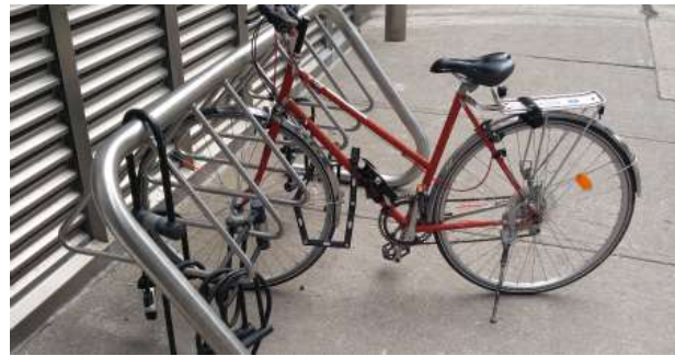
Figure 9.12 – Coat-hanger Rack (Not Preferred for Most Situations)
