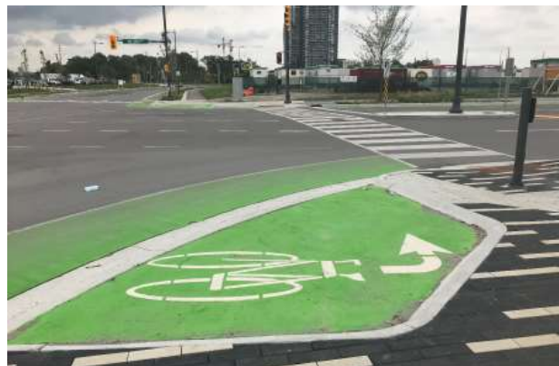
Figure 6.46 – Example of In-Boulevard Two-Stage Queue Box, Vaughan
