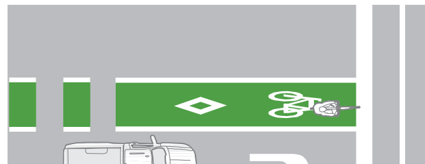
Figure 6.12 – Solid Green Treatment on Intersection Approach
